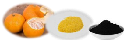
Figure 1. Synthesis of porous carbon from tangerine peels
