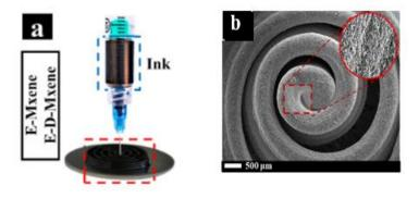
Figure 1. Illustration of 3D MXene ink printed electrodes with different layers.
