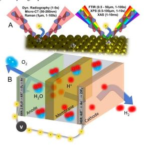
Figure 1. Schematic of artist rendering of (A) *Operando* techniques with their temporal and spatial resolutions. (B) Main electrolysis reactions and a typical system cell structure [3].
