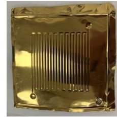
Figure 3. Ti interlayer TiN coated serpentine air funnel BPP.
