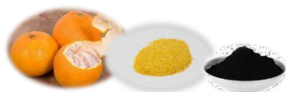
Figure 1. Synthesis of porous carbon from tangerine peels
