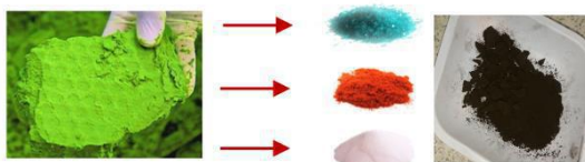
Figure 1. MHP product and produced sulfate salts (nickel, cobalt and manganese sulphate respectively) and CAM
